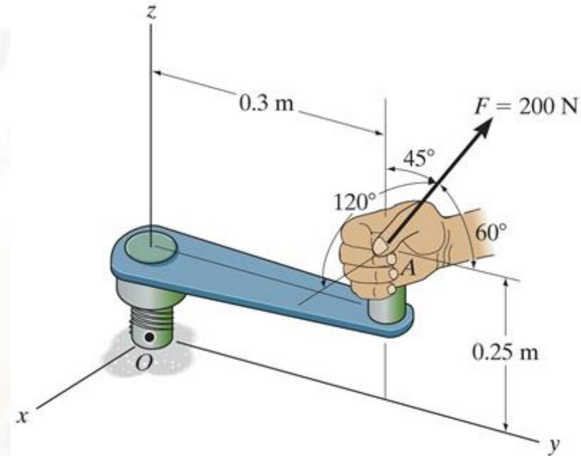
3. The force  $F$  acts on a bracket as shown in the figure. Take  $\alpha = 60^\circ$ ,  $\beta = 60^\circ$ ,  $\gamma = 45^\circ$ . Find the magnitude of the moment about a-a axis.
